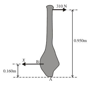
One horizontal force is missing from the diagram. Add an arrow to represent this force and label it *Y*.
