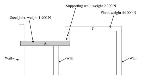
The steel joist A supports the supporting wall B and the left-hand side of floor C. Both the joist and floor C may be treated as uniform bars.
