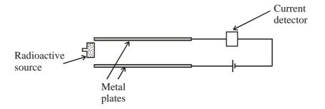
Radiation from the source ionises the air between the plates, and a small current is detected. If smoke enters the detector, the ions 'stick' to the smoke particles, reducing the current and triggering an alarm.
