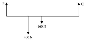
Calculate the tension in each suspended wire.
