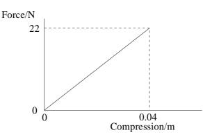
Calculate the work done on the spring when it is compressed by 4.0 cm.
